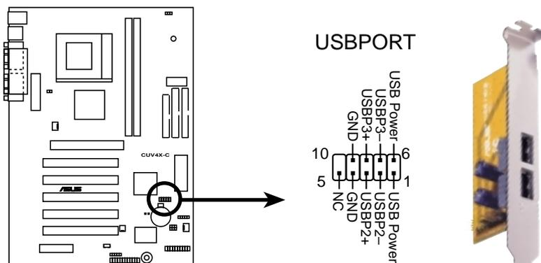
**CUV4X-C Front Panel USB Header**
