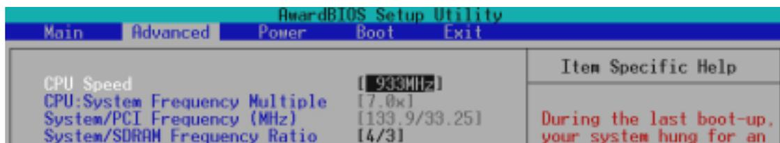
**Cause for Hangup: Improper CPU Speed**
