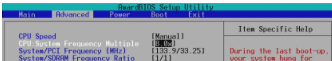
**Cause for Hangup: Improper CPU: System Frequency Multiple (For processors with unlocked frequency multiplier only)**
