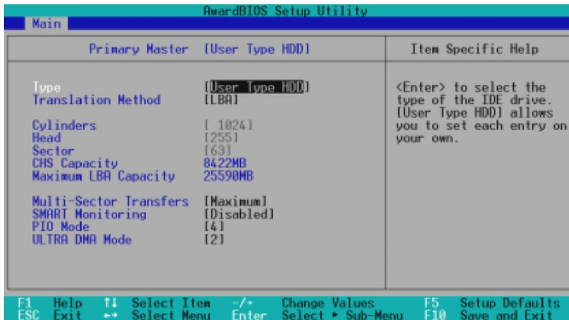
Manually enter the number of cylinders, heads and sectors per track for your drive. Refer to your drive documentation or look on the drive for this information. If no drive is installed or if you are removing a drive and not replacing it, select [None].
