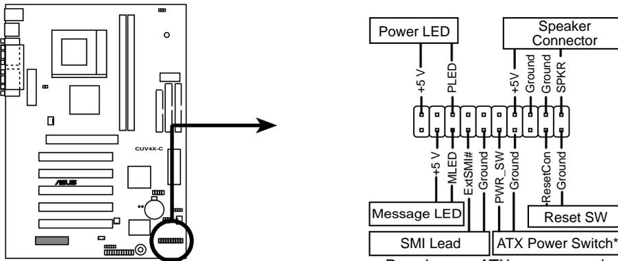
**CUV4X-C System Panel Connectors**
