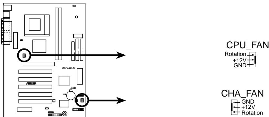
**CUV4X-C 12-Volt Cooling Fan Power**
