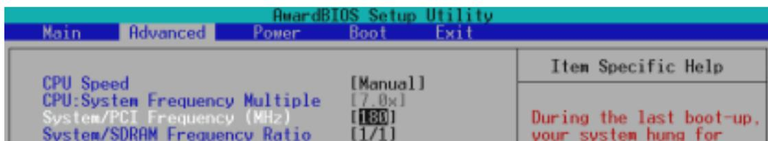
**Cause for Hangup: Improper System/SDRAM Frequency Ratio**
