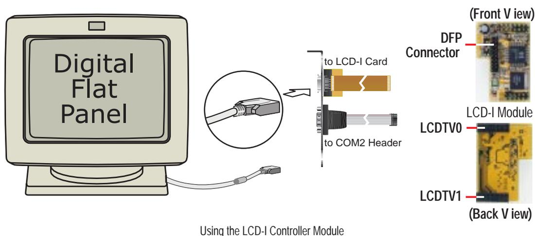
**NOTE:** The LCD-I controller module can work with your LCD panel without any driver. However, if you want to have full-screen display, please set up the VGA driver that comes with your motherboard's support CD.
