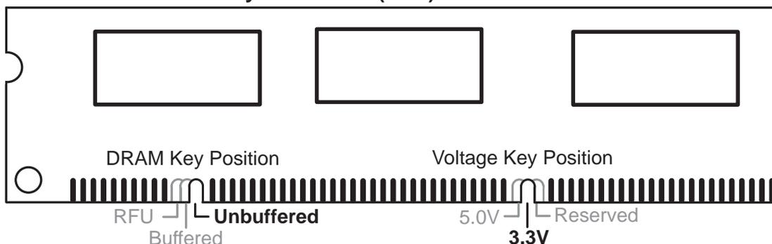
The notches on the DIMM will shift between left, center, or right to identify the type and also to prevent the wrong type from being inserted into the DIMM slot on the motherboard. You must ask your retailer the correct DIMM type before purchasing. This motherboard supports four clock signals per DIMM slot.
