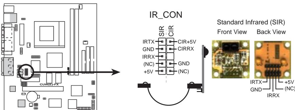
**CUW(E)-FX Infrared Module Connector**
