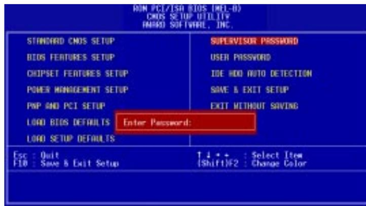
To implement password protection, specify in the “Security Option” field of the BIOS Features Setup screen when the system will prompt for the password. If you want to disable either password, press <Enter> instead of entering a new password when the “Enter Password” prompt appears. A message confirms the password has been disabled.
