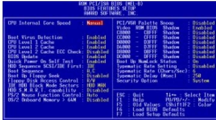
A section at the lower right of the screen displays the control keys you can use. Take note of these keys and their respective uses. If you need information on a particular entry, highlight it and then press <F1>. A pop-up help menu will appear to provide you with the information you need. <F5> loads the last set values, <F6> and <F7> loads the BIOS default values and Setup default values, respectively.
