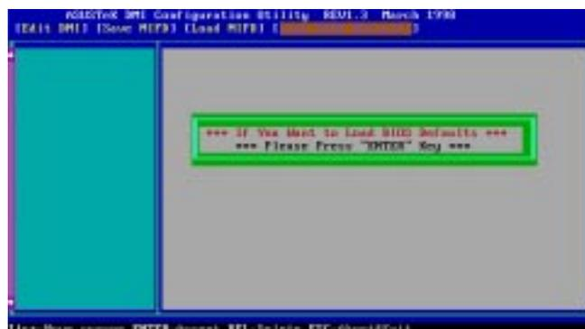
You can load the BIOS defaults from a MIFD file and can clear all user modified and added data. You must reboot your computer in order for the defaults to be saved back into the Flash BIOS.
