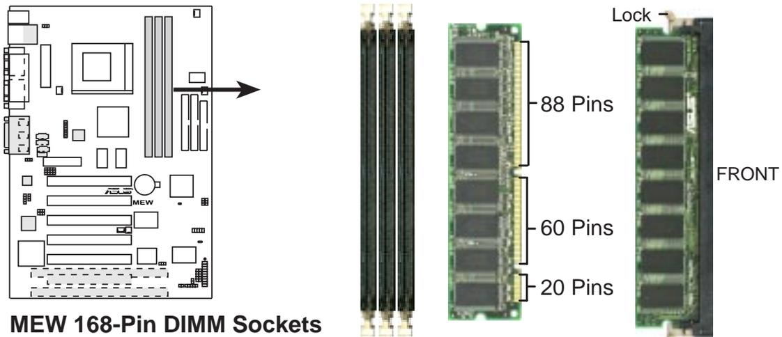
The DIMMs must be **3.3V Unbuffered** for this motherboard. To determine the DIMM type, check the notches on the DIMMs (see figure below).
