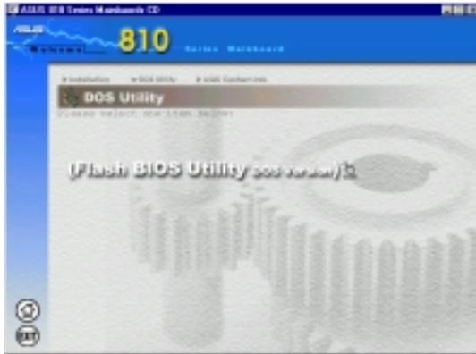
**Flash BIOS Utility (DOS Version):** Provides information on the Flash BIOS utility (AFLASH.EXE). Choose “Restart in MS-DOS mode” then type “aflash” from the AFLASH folder on the support CD.
