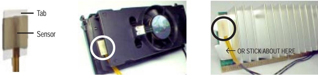
**WARNING!** Do not insert the sensor between the processor and heatsink, otherwise, it will cause damage to the P2T-Cable.
