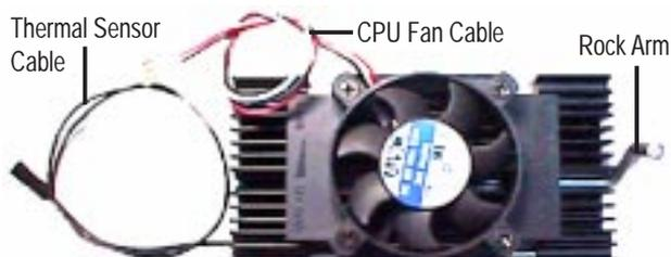
an integrated thermal sensor located near the center of the CPU heat source. The sensor is optimized by ASUS to give the most accurate reading of the CPU temperature, thus provides the best protection to your computer system.
