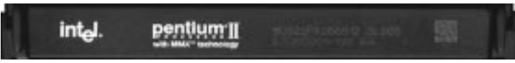
Intel Pentium II Processor in a SEC Cartridge (233-333MHz 512KB/256KB/0KB L2 Cache)
