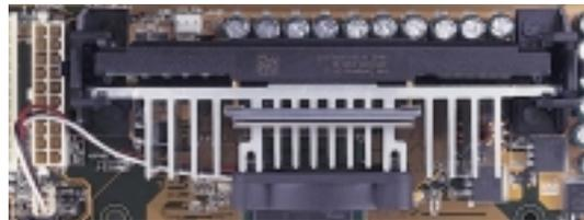
Pentium III (in an SECC2) with heatsink and fan
