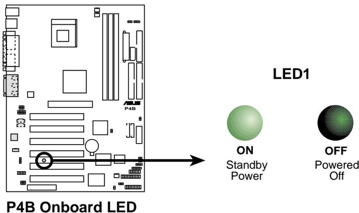
Figure 2-3 Onboard Power LED
