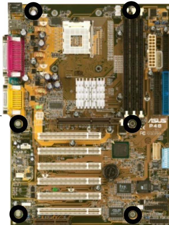
Figure 2-1 Motherboard placement and screw holes
