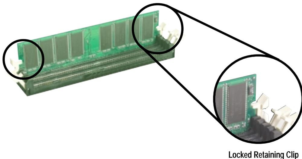
Figure 2-15 Installed DIMM
