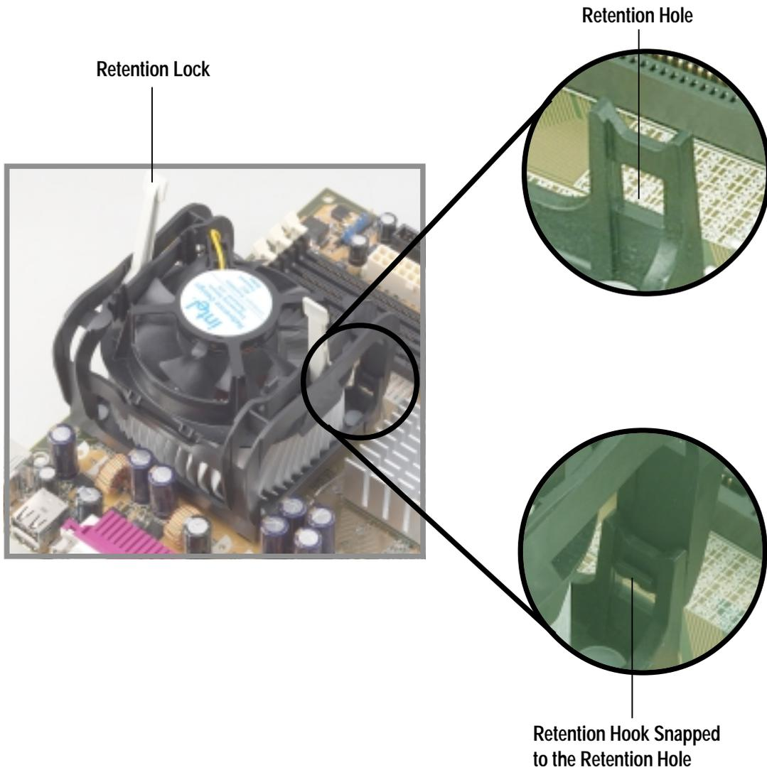
*Figure 2-10 Installing the Fan and Retention Mechanism*
