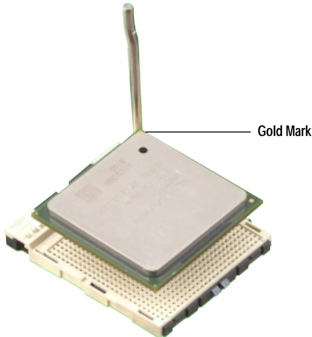
*Figure 2-7*      *Installing the CPU*
