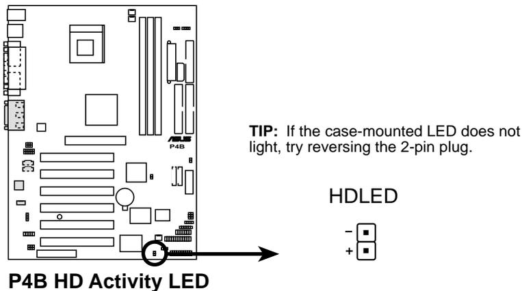
Figure 2-31 Hard Disk LED Connector
