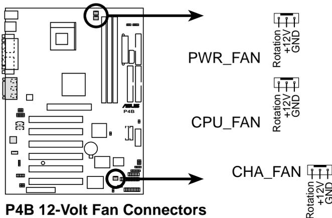
Figure 2-35 CPU, Chassis, and Power Fan Connectors
