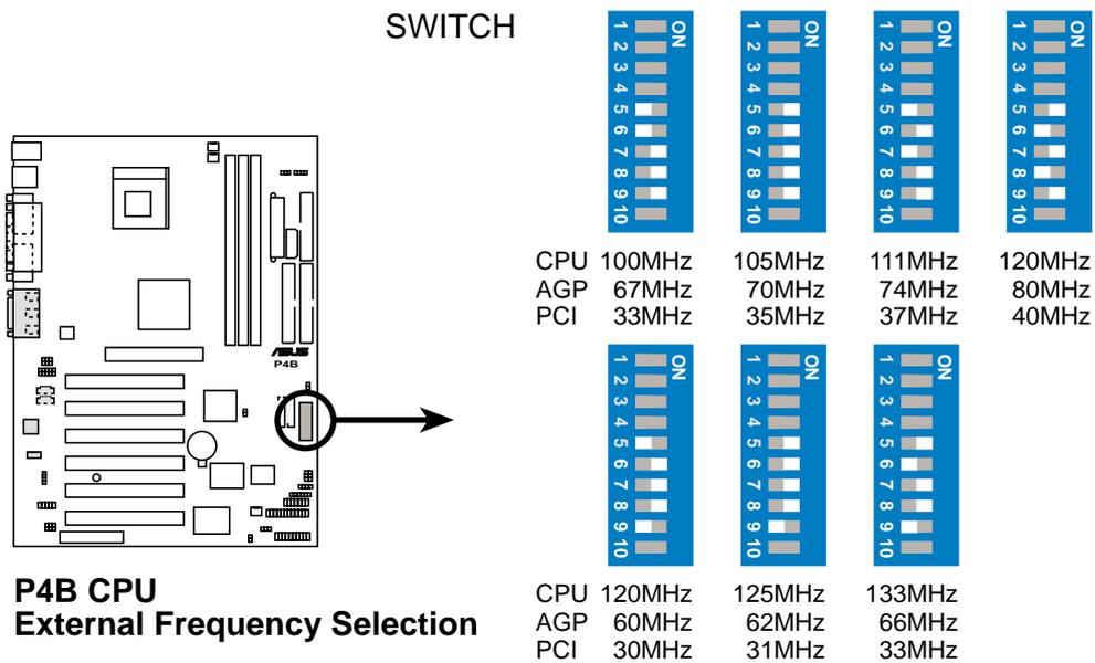
Figure 2-24 CPU Frequency Settings
