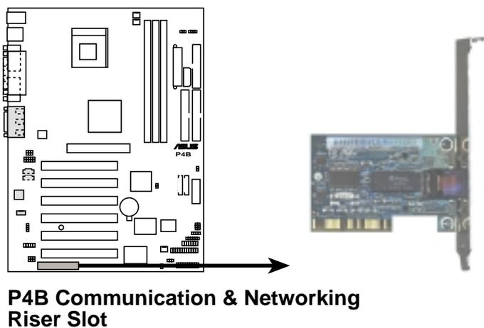
*Figure 2-20*      *Communications and Networking Riser (CNR) Slot Location*
