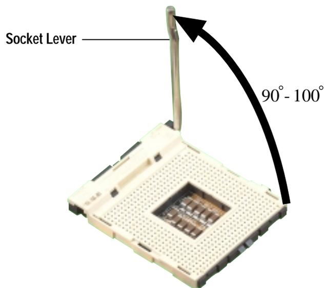
Figure 2-6 CPU Socket Lever at 90° - 100° Angle
