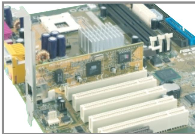
Figure 2-18 Installed PCI Card
