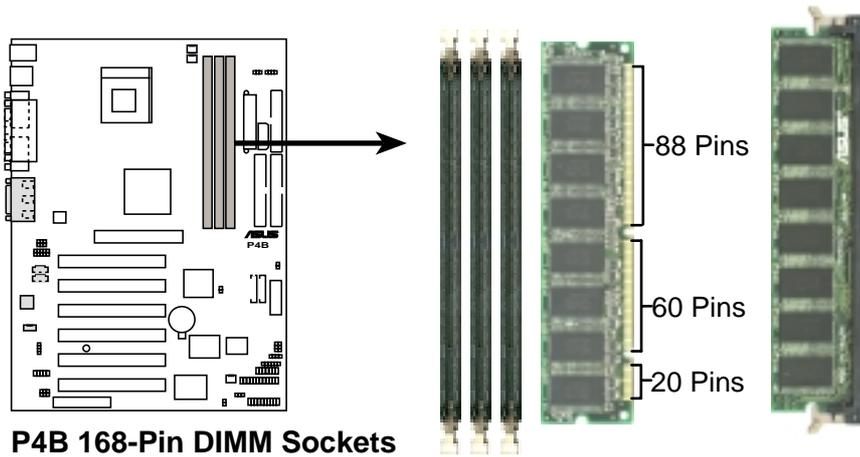
Figure 2-13 DIMM Sockets Location and SDR DIMMs
