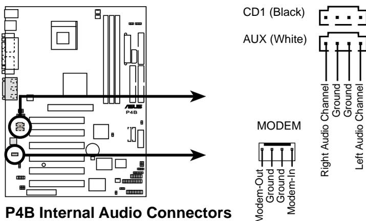
Figure 2-39 Internal Audio Connectors
