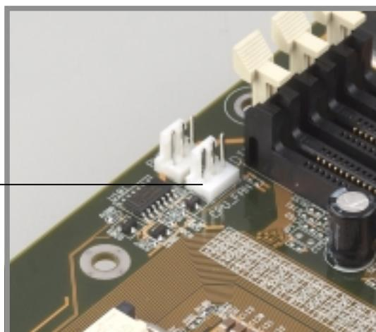
Figure 2-12 CPU Fan Connector
