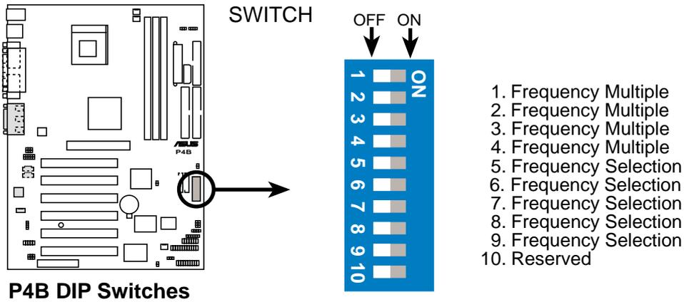
Figure 2-21 DIP Switches
