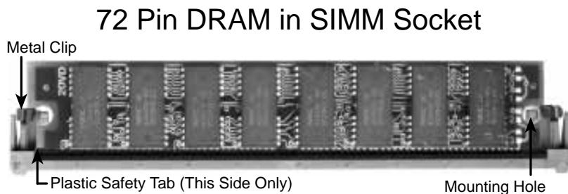
4. The plastic guides should go through the two "Mounting Holes" on the sides and the "Metal Clips" should snap on the other side.
