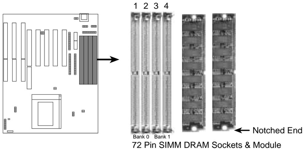
2. Press the memory module firmly into place starting from a 45 degree angle making sure that all the contacts are aligned with the socket.
