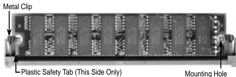
4. The plastic guides should go through the two "Mounting Holes" on the sides and the "Metal Clips" should snap on the other side.
