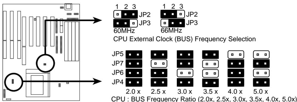
Set the jumpers by the Internal speed of the Intel CPU as follows:
