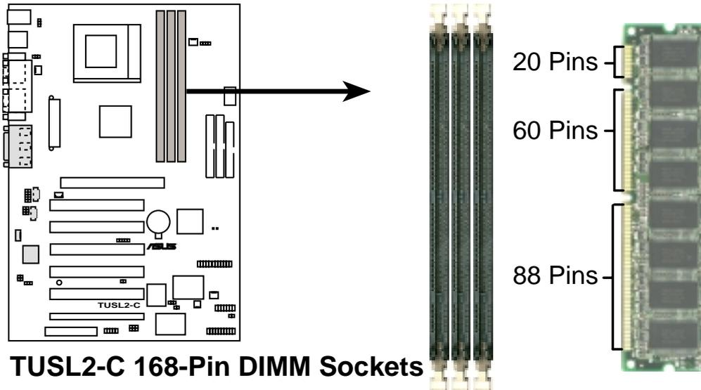
The DIMMs must be 3.3Volt unbuffered SDRAMs. To determine the DIMM type, check the notches on the DIMMs (see figure below).
