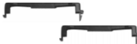
NOTE: For the retention mechanism and lock bar, there is a left and a right side. The left side has a single dot and the right side has two dots (when holding the motherboard with the ATX connectors to the left).
