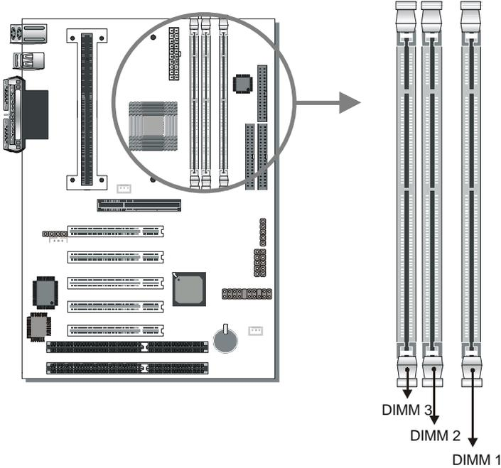
Your board comes with three DIMM sockets, providing support for up to 768MB of main memory using unbuffered DIMM modules from 8MB to 256MB. PC100 DIMM module is required on this motherboard.
