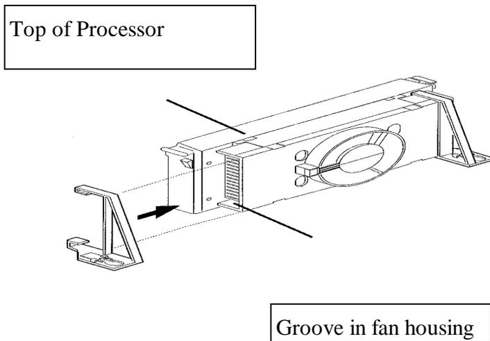
3. Slide the clip (A) on each support toward the processor , exposing the hole that will fit the peg on the mainboard . Push the latches (B) on the processor toward the center of the processor until they click into place.
