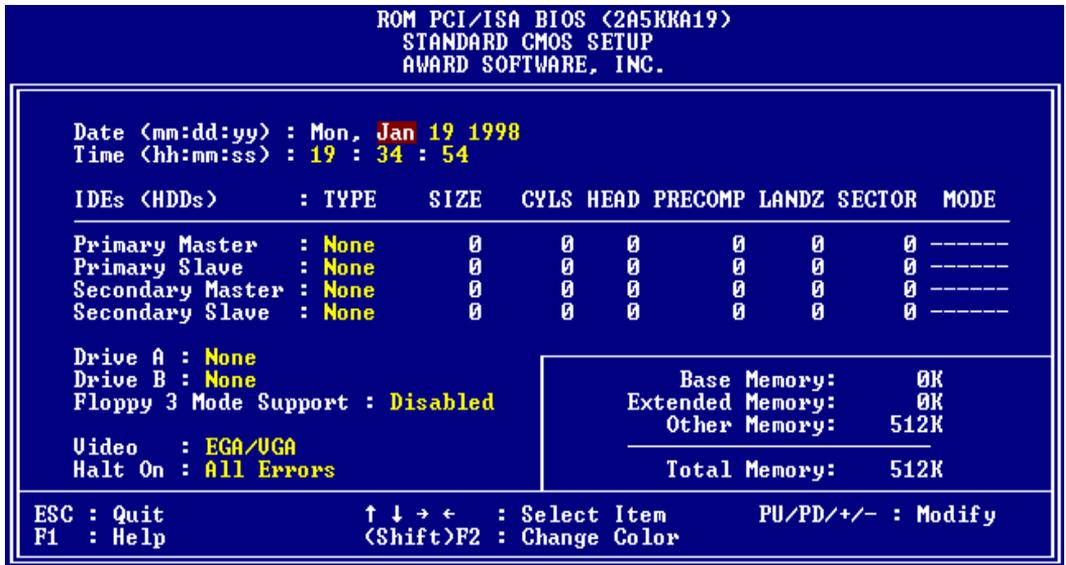
Fig 3-2 Standard CMOS Setup Menu
