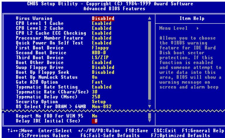
Figure 3-5. Advanced BIOS Features Setup
