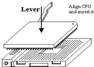
Figure 2-4. Install the CPU into socket 370
