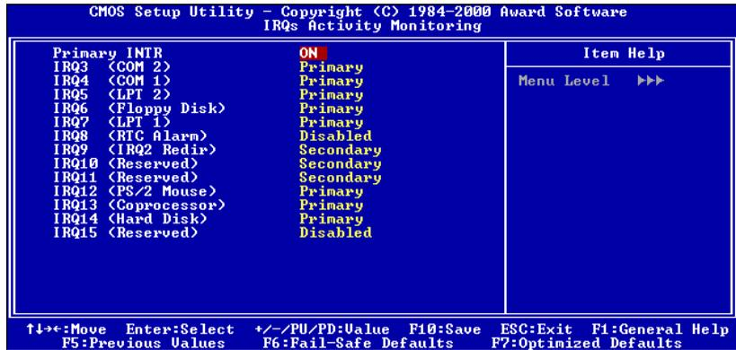
**Figure 3-7D. IRQs Activity Monitoring Setup Menu****Primary INTR:**
