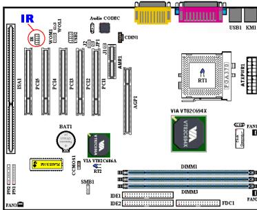
There is a specific orientation for pins 1 through 5, attach the connector from the IR KIT or IR device to the IR1 header (left row only). This motherboard supports standard IR transfer rates.
