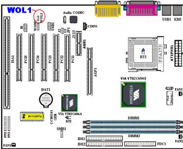
If you have a network adapter that supports this feature, then you can connect the specific cable from the network adapter to this header. This feature lets you wake up your computer via remote control through a local area network. You may need a specific utility to control the wake up event, like using the PCnet Magic Packet utility or other similar utilities.
