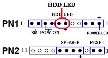
Attach the cable from the case's front panel HDD LED to this header. If you install it in the wrong direction, the LED light will not illuminate correctly.
