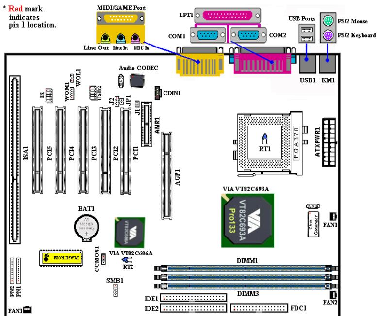
Figure 1-2. VL6 Motherboard component location
