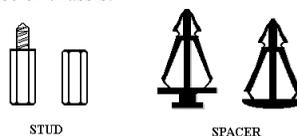
Figure 2-1. The outline of stud and spacer
