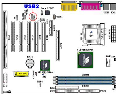
This header is for connecting the additional USB ports plugs. You can use the special USB port extend cable (option), it can provides you additional two USB plugs, you can fix these USB plugs on the back panel.
