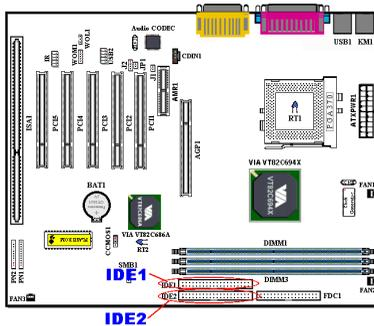
An IDE hard disk drive ribbon cable has 40 wires and two connectors to provide a connection for two IDE hard disk drives. After connecting the single end to the IDE1 (or IDE2), connect the two connectors on the other end to the IDE hard disk drives (or CD-ROM drive, LS-120, etc.).
