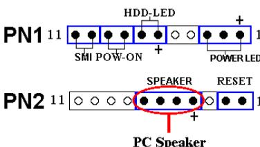
Attach the cable from the system speaker to this header.
