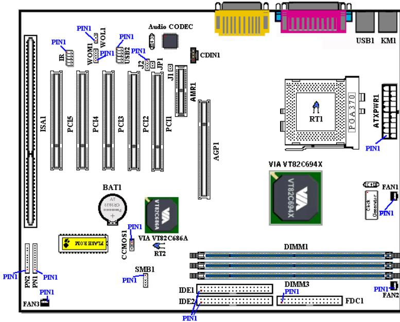
Figure 2-7. All Connectors and Headers for the VL6
