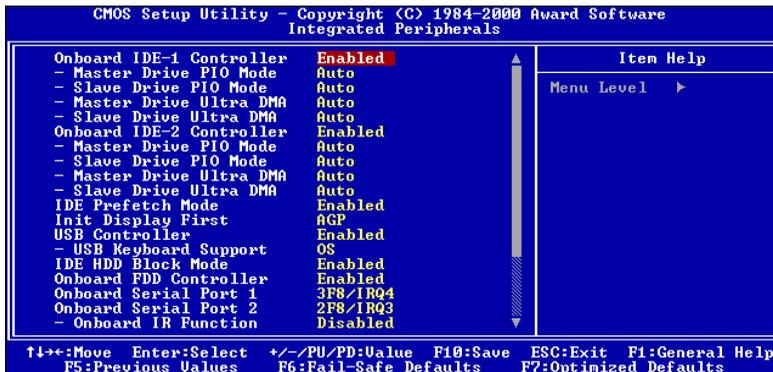
Figure 3-6A. Integrated Peripherals Menu Upper Screen
