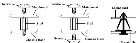
Figure 2-2. The way we fixed the motherboard
