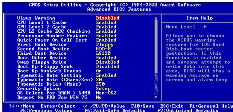
Figure 3-4A. Advanced BIOS Features Setup Upper Screen
