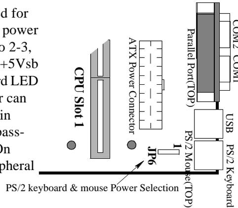
**JP6 shunt 1-2:** PS/2 keyboard & mouse use power supply's +5V.
