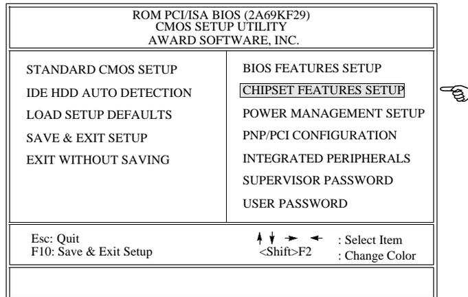
2) On the top right hand side of the “Chipset Feature Setup” screen, there is a “CPU Speed” option. Refer to the table below and select the correct CPU speed.
