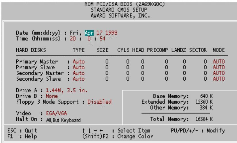
Figure 4.2: Standard CMOS Setup Menu
