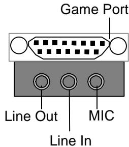
Line Out 1: Line Out or SPDIF (The SPDIF output is capable of providing digital audio to external speakers or compressed AC3 data to an external Dolby digital decoder). In general, Line Out 1 is normally Line Out, when it output digital signal, it will be change to SPDIF Out automatically (see page 39 for more information).
