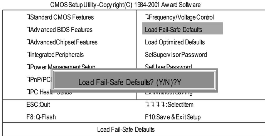
Figure 11: Load Fail-Safe Defaults
