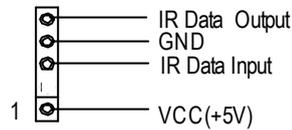
⚠ Be careful with the polarity of the IR connector while you connect the IR. Please contact your nearest dealer for optional IR device.
