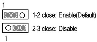
⚠ This MB supports optional LAN chip. If the MB has optional LAN chip the user can enable the LAN function by setting the "LAN\_EN" to 1-2, user can disable the optional LAN function by setting the "LAN\_EN" to 2-3. "LAN\_EN" will have any effect if the board does not have optional LAN chip.
