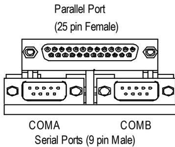
⚡ This connector supports 2 standard COM ports and 1 Parallel port. Device like printer can be connected to Parallel port ; mouse and modem etc can be connected to Serial ports.
