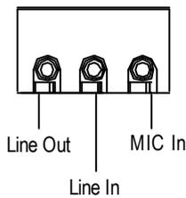
☞ After install onboard audio driver, you may connect speaker to Line Out jack, micro phone to MIC In jack. Device like CD-ROM , walkman etc can be connected to Line-In jack.
