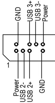
⚠ Be careful with the polarity of the front panel USB connector. Check the pin assignment while you connect the front panel USB cable. Please contact your nearest dealer for optional front panel USB cable.
