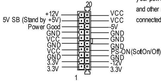
⚠ AC power cord should only be connected to your power supply unit after ATX power cable and other related devices are firmly connected to the mainboard.
