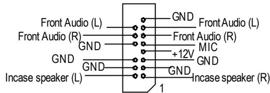
⚠ If you want to use "Front Audio" connector, you must move 11-12, 13-14 Jumper. In order to utilize the front audio header, your chassis must have front audio connector. Also please make sure the pin assignment on the cable is the same as the pin assignment on the MB header. To find out if the chassis you are buying support front audio connector, please contact your dealer.
