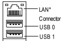
☞ Before you connect your device(s) into USB connector(s), please make sure your device(s) such as USB keyboard, mouse, scanner, zip, speaker..etc. Have a standard USB interface. Also make sure your OS (Win 95 with USB supplement, Win98, Windows 2000, Windows ME, Win NT with SP 6) supports USB controller. If your OS does not support USB controller, please contact OS vendor for possible patch or driver upgrade. For more information please contact your OS or device(s) vendors.
