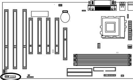
The 2-pin IDE LED header is located on pins 5--6 (identified as ALED). Connect the cable from ALED header to the LED on the front panel of your PC case.
