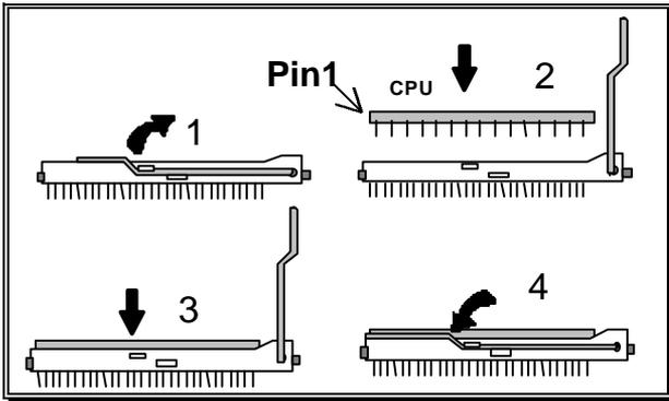
Follow this quick four-step process to install the CPU:
