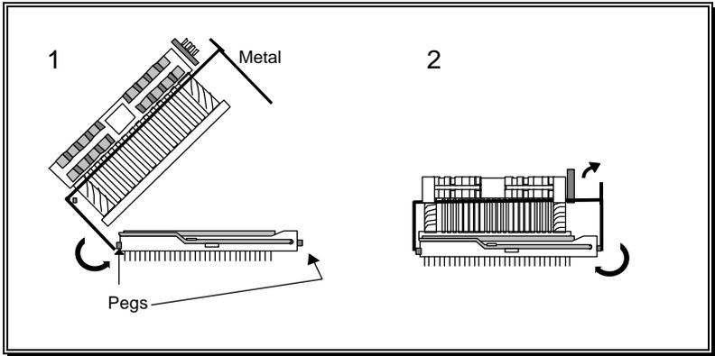
Follow this two-step process to install CPU fan:
