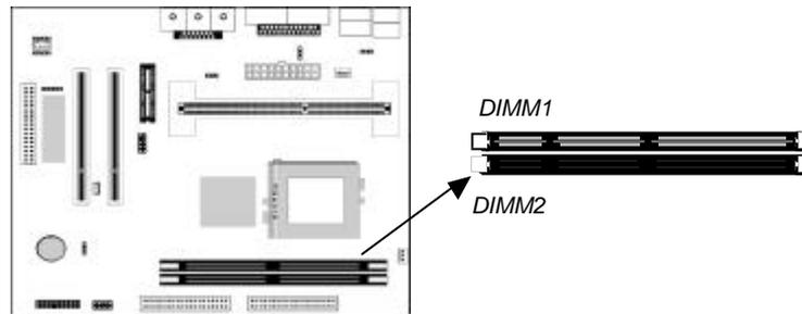
For this mainboard, you must use 168-pin, 3.3V unbuffered SDRAM memory modules. If the installed CPU uses a 100MHz system bus, you must use PC100 or PC133 memory. If the installed CPU uses a 66MHz system bus, you must use PC66 memory. You can install any size memory module from 16 MB to 512MB, so the maximum memory size is  $2 \times 512\text{MB} = 1\text{GB}$ .
