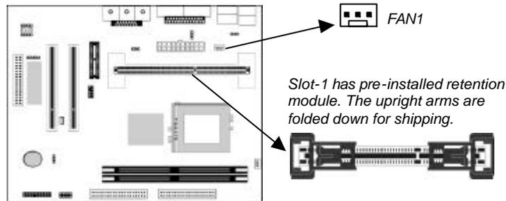
2. The Slot-1 is installed with a retention module. The upright arms of the module are folded down for shipping. Raise the arms so that they are in the upright position.
