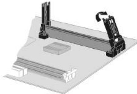
3. Slide the CPU cartridge into the module arms. Follow the instructions that come with the CPU. The edge connector on the CPU cartridge has a notch so that it only fits into the Slot-1 in the correct way.
