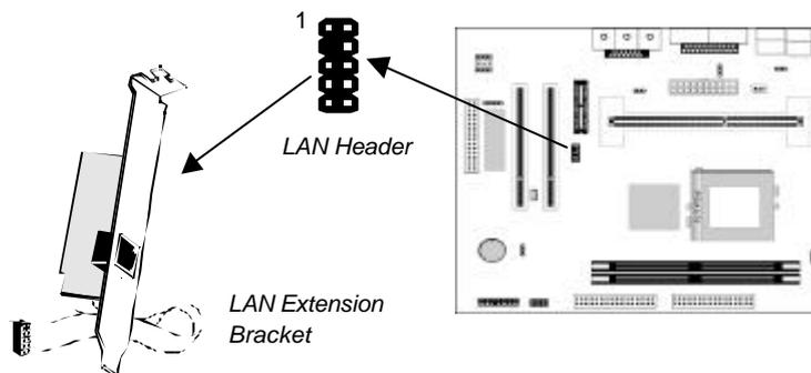
1. On the mainboard, locate the LAN header for this bracket.
