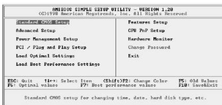
You can use the cursor arrow keys to highlight any of the options on the main menu page. Press **Enter** to select the highlighted option. To leave the setup utility, press the **Escape** key. To cycle through the Setup Utility's optional color schemes hold down the **Shift** key and press **F2**.
