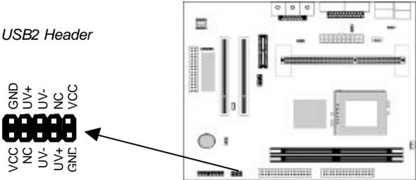
1. Locate the **USB2** header on the mainboard.
