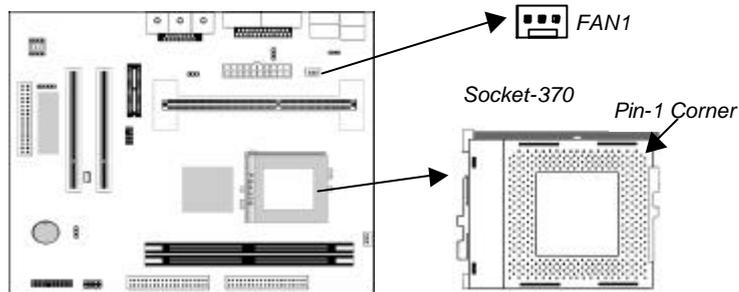
2. On the processor, identify the Pin-1 corner by its beveled edge.
