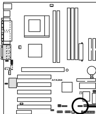
**A7A266 Chassis Open Alarm Lead**
