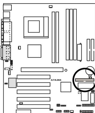
**NOTE:** Orient the red markings on the floppy ribbon cable to PIN 1
