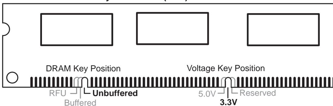
The notches on the DIMM will shift between left, center, or right to identify the type and also to prevent the wrong type from being inserted into the DIMM slot on the motherboard. You must tell your retailer the correct DIMM type before purchasing. This motherboard supports four clock signals.
