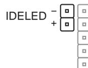
**TIP:** If the case-mounted LED does not light, try reversing the 2-pin plug.
