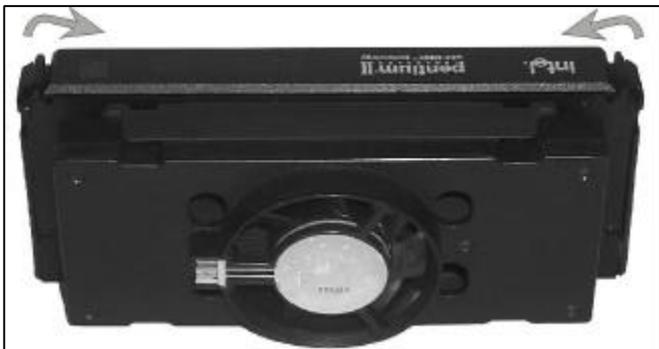
3. Insert the CPU into the retention module. The CPU fits in the CPU slot in only ONE way, do not try to force it in.
