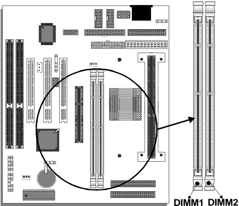
Your board comes with two DIMM sockets, providing support for up to 256MB of main memory using DIMM modules from 8MB to 128MB with no restriction on memory configuration. Therefore, you can install memory modules in any combination.
