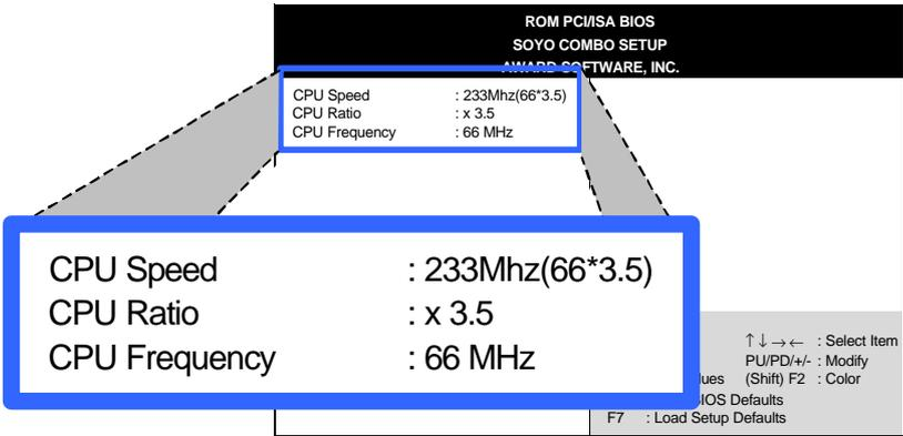
Available [CPU Speed] settings on your SY-6IEB Mainboard are detailed in the following table. If you set this field to [Manual], you are then required to fill in the next two consecutive fields: (1) the CPU Ratio, and (2) the CPU Frequency.
