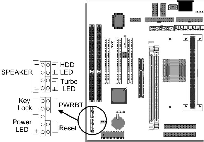
Plug the computer case's front panel devices to the corresponding headers on the mainboard.
