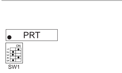
Figure 2-1-1. CPU Jumper Settings
