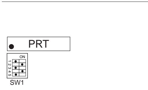
Figure 2-1-3. CPU Jumper Settings
