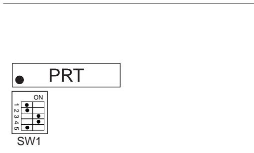
Figure 2-1-4. CPU Jumper Settings
