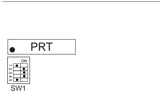
Figure 2-1-2. CPU Jumper Settings
