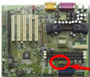
This jumper is used to specify the relationship of PCI and CPU Bus clock. Generally speaking, if you are not overclockers, we recommend to set at the default setting.
