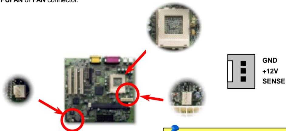
**Note:** Some CPU fans do not have sense pin, so that cannot support fan monitoring.
