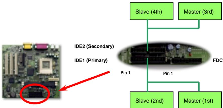
IDE1 is also known as the primary channel and IDE2 as the secondary channel. Each channel supports two IDE devices that make a total of four devices. In order to work together, the two devices on each channel must be set differently to **master** and **slave** mode. Either one can be the hard disk or the CDROM. The setting as master or slave mode depends on the jumper on your IDE device, so please refer to your hard disk and CDROM manual accordingly.
