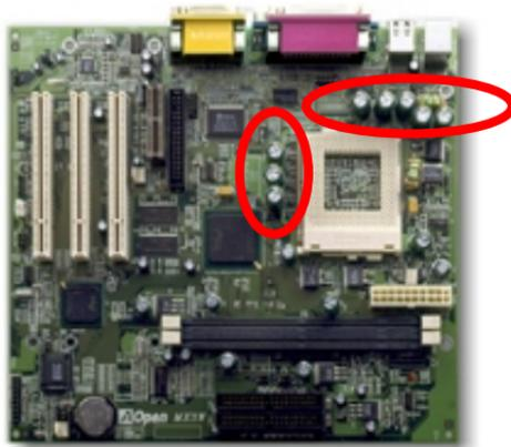
The power circuit of the CPU core voltage must be checked to ensure system stability for high speed CPUs (such as the new Pentium III, or when overclocking). A typical CPU core voltage is 2.0V, so a good design should control voltage between 1.860V and 2.140V. That is, the transient must be below 280mV. Below is a timing diagram captured by a Digital Storage Scope, it shows the voltage transient is only 143mV even when maximum 18A current is applied.
