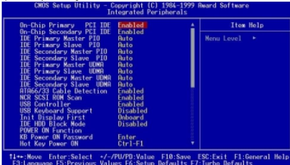
This page is the lower half of Integrated Peripherals submenu.
