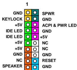
Attach the power LED, keylock, speaker, and reset switch connectors to the corresponding pins. If you enable Power Management > [ACPI Function](#) in BIOS Setup, the ACPI & Power LED will keep flashing while the system is in suspend mode.
